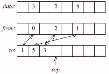
The variable top is initially zero; the array element i is first accessed by the code
